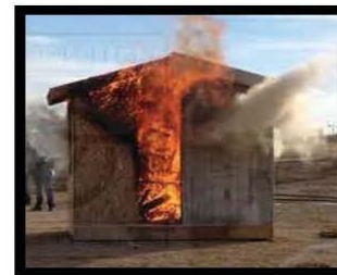
Fire Test of OSB + Closed Cell Polyurethane + OSB SIP vs TGS SIP The OSB had a 2.5-hour fire rating, using Fire-Retardants.
